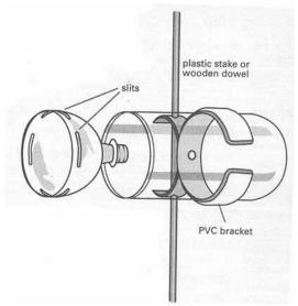
Figure 2. Activity trap design illustrating adjustable PVC bracket and funnel grooves.
