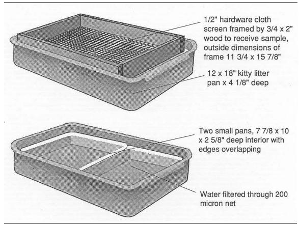
Figure 1. Diagram of hardware cloth and tray apparatus for separating invertebrate specimens from vegetation collected in dip net samples.
