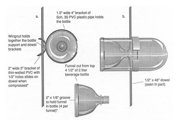
Figure 3. Activity trap design illustrating a) view into funnel and b) lateral view.
